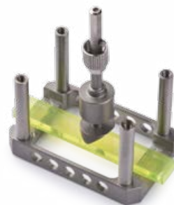
Sample holder for 3-point bending
