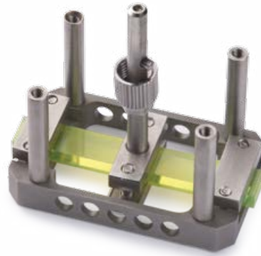
Sample holder for dual cantilever bending
