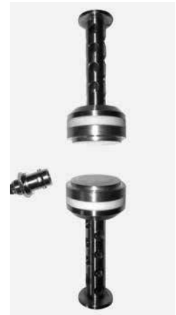
Dielectric dynamic-mechanical combination
