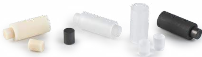
Sample containers made of alumina, sapphire and graphite for measurements on powders, pastes and liquids
